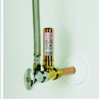
Stop Valve Connection Unique fitting installs between \frac{3}{8} " Compression stop and supply tube, or between stub out and \frac{5}{8} " Compression stop
